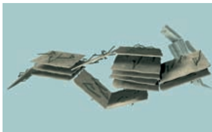
Incomplete dispersion of organo clay platelets
