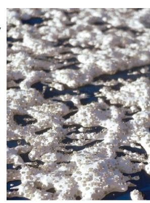
Reflective glas beads on top of a DEGAROUTE® based road marking
